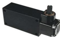
3 Way Normally Closed Max psi: Air Temp range: 32° to 230°F Travel Arc: 0-23 off 23-50 on Flow: 10 cfm @ 100 psi Force: 3"/lbs
