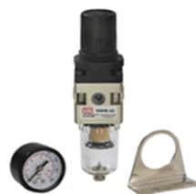
19 cfm With auto drain Medium: Air Temp range: 32° to 150°F Flow: 19 scfm at 100 psi Seals: Buna-N 25 Micron Filter
